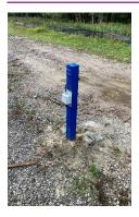
**SAFETY FACT:** We installed analytical instruments called Pizeometers and Inclinometers at the Edenville Dam embankment while SCB cutoff wall work progresses. These sensitive instruments detect slight changes in water pressure and movement of the embankment while the heavy equipment is trenching on the crest allowing the work to be done safely and without damaging the earth filled embankment.
