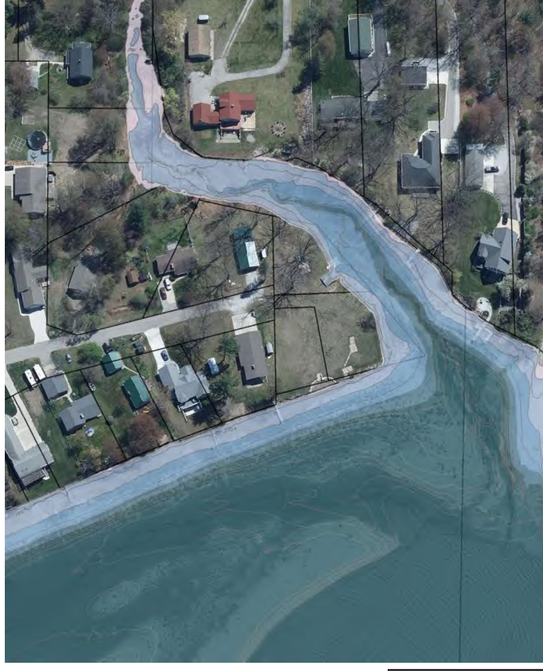
Sanford Lake - Depth data from 2020 Q1 LIDAR, captured June 1, 2020.
